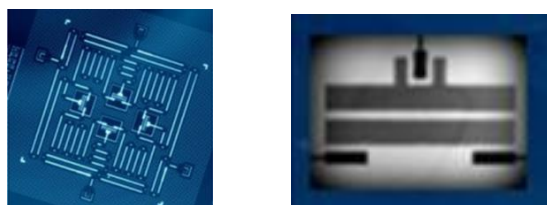
Fig. 10 Network of four qubits (left) of IBM Quantum Experience. An electron microscope picture of a JJ qubit (right).
